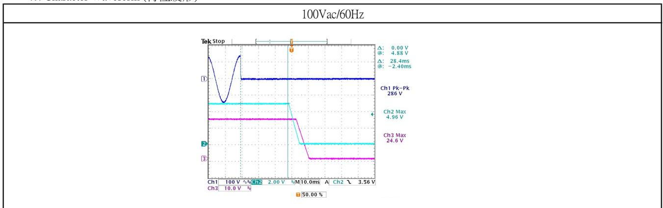
2-2. Low Vac Shut Off (輸入欠壓關斷特性)
